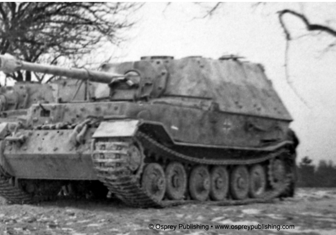
After completion, the Ferdinands, now renamed Elefant , were parked on a field near the Nibelungenwerke. Note the vehicles now have a self-defence Maschinengewehr 34 (MG 34) and are coated with Zimmerit anti-magnetic mine paste. (Historyfacts)
