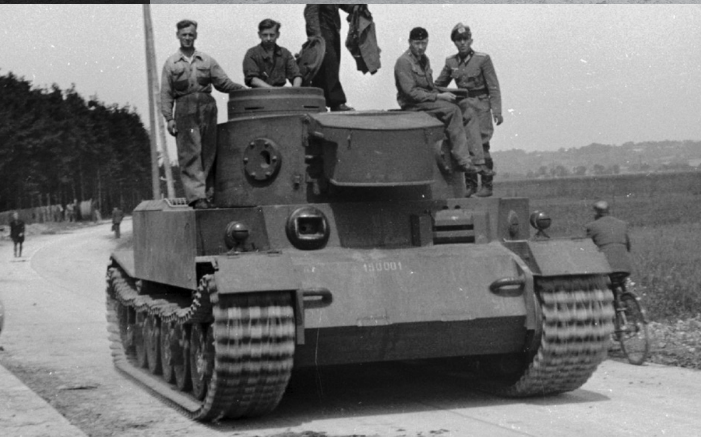
Porsche No.150001 on trials: Despite the vehicle's number, this was not the first of the type to be completed. A PzKpfw IV-type Gepäckkasten (stowage bin) is fitted on the rear of the turret. (Historyfacts)
