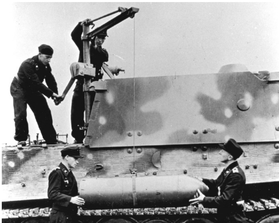
The crew of a Sturmörser carefully loads a massive 38cm rocket shell using a turret-mounted gantry crane. The tank is painted in the Licht-und-Schatten Tarnung (Light and Shadow camouflage), also known as the ambush scheme. (Historyfacts)
