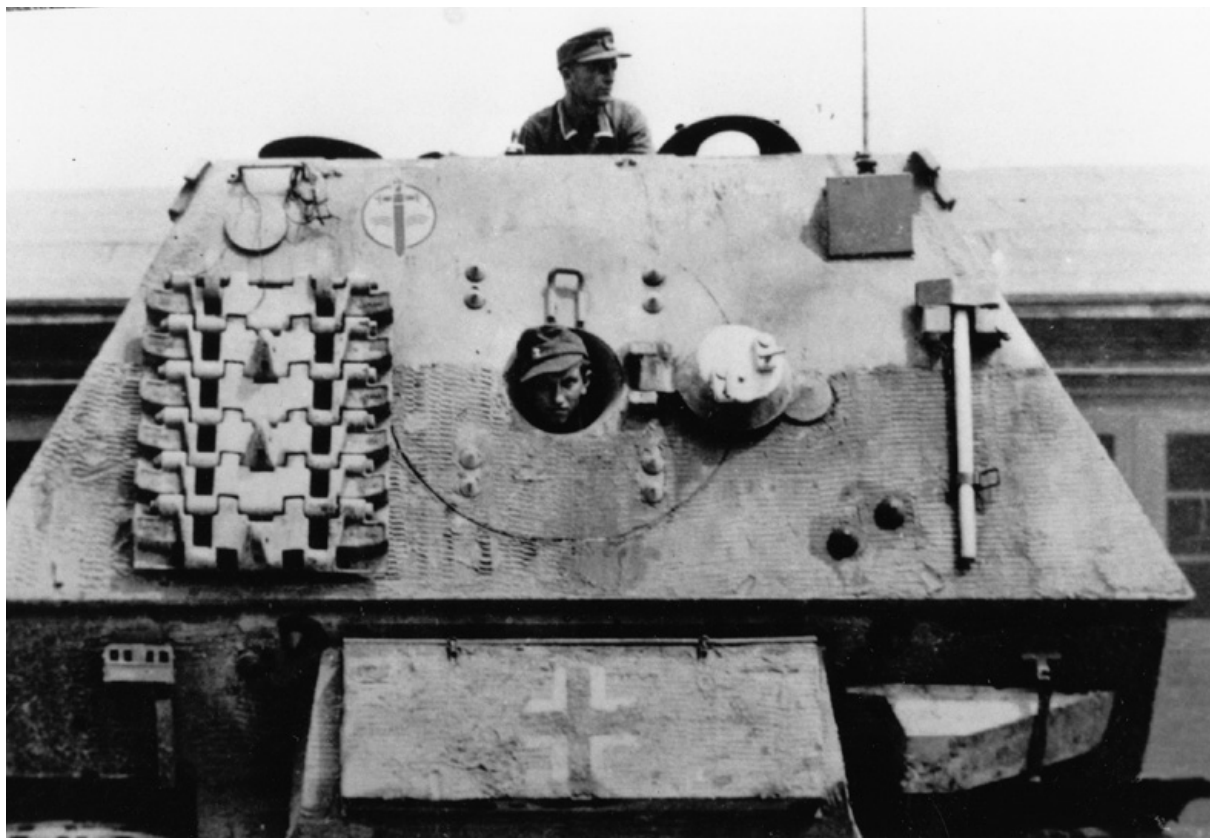
An Elefant fitted-out as a command tank, note the second radio antenna mounted on the rear of the vehicle. The large box mounted on the exhaust cover contained the gun-cleaning kit. (Schneider)
