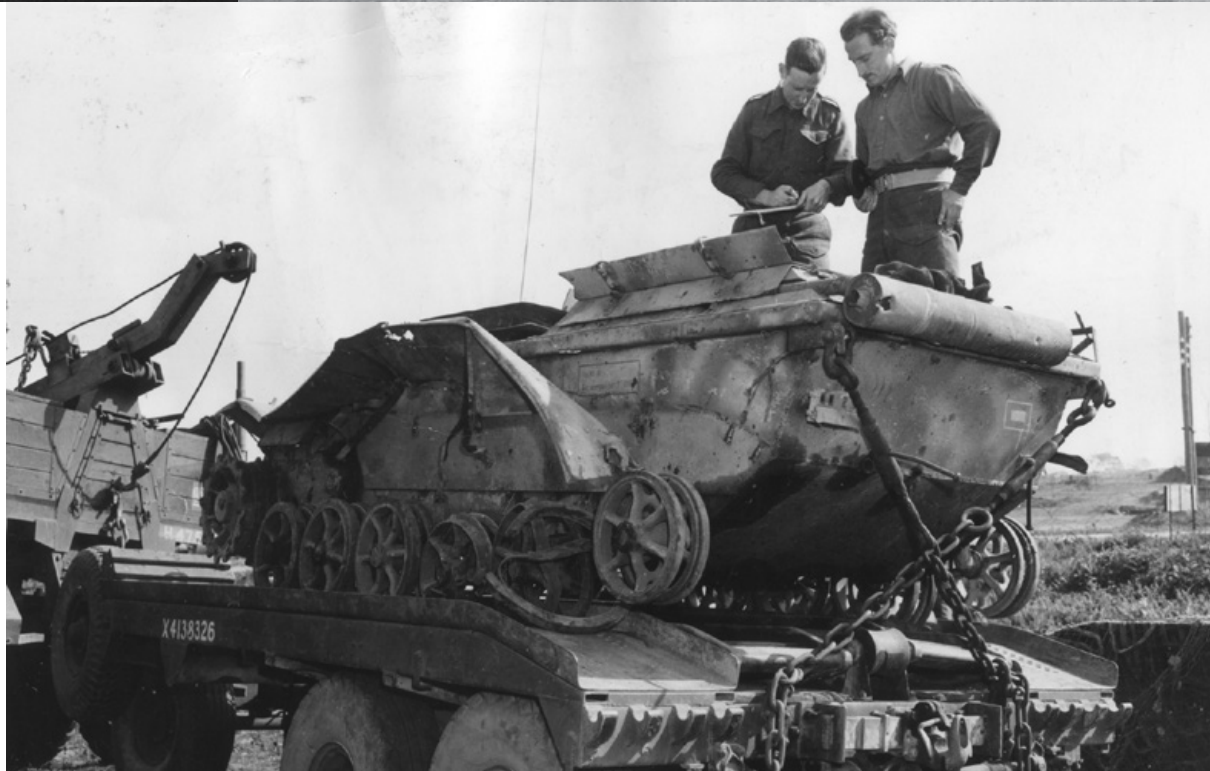
A Borgward B IV from PzAbt (Fk) 301 captured by British troops near Nettuno, Italy, is loaded on a transport vehicle to be taken away for evaluation. The tracks are badly damaged due, probably, to the vehicle being guided in to clear a minefield. The bay for the 450kg explosive charge is empty. (NARA)
