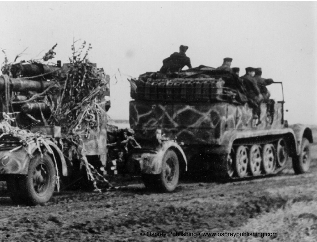
An 8.8cm Fliegerabwehrkanone 36 (8.8cm FlaK 36) towed by an SdKfz 7 half-track vehicle passes engineers working to repair a Ferdinand. (PK photo)
