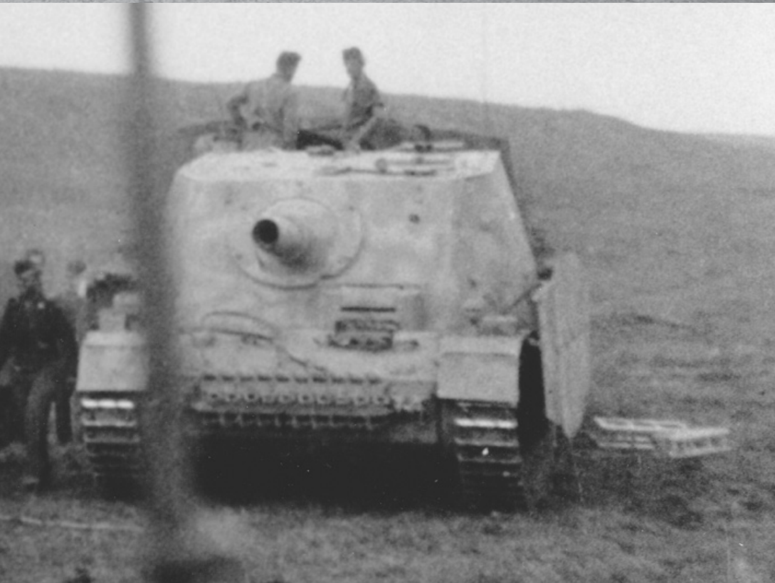
A Sturmpanzer of StuPzKp 216. This vehicle was built on the chassis of a refurbished PzKpfw IV Ausf E hull, as evident by the bolted-on armor plate. (Jaugitz)
