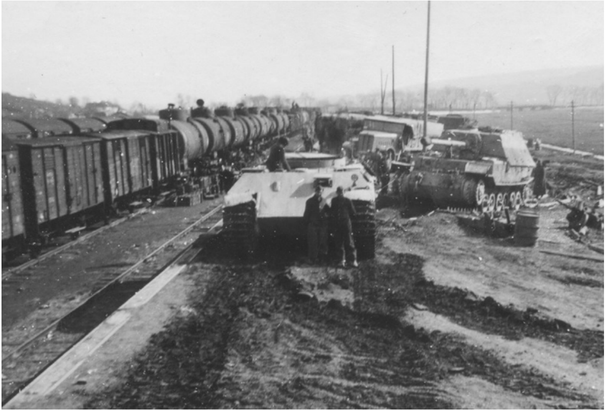
Loading damaged Elefants onto a railway wagon was a very difficult task, and almost impossible without a head ramp. A Bergepanther is being used to haul a trackless Elefant nearer to the loading platform. (Anderson)
