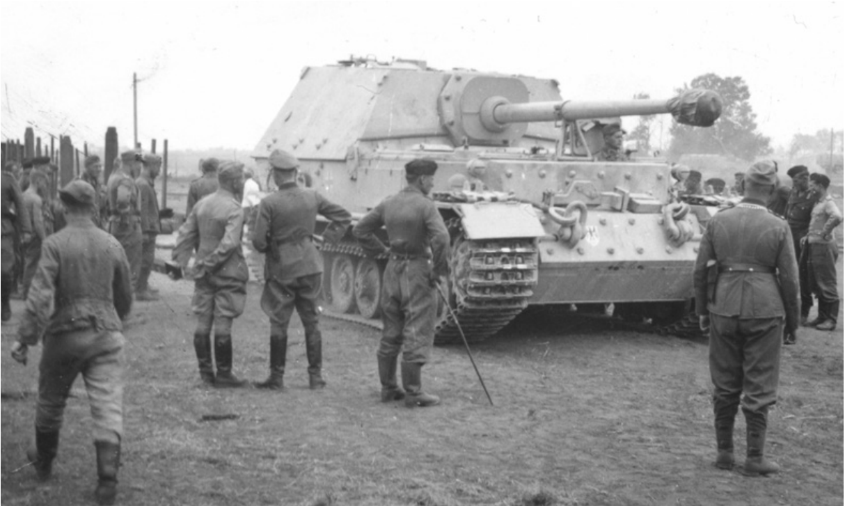
A vehicle from sPzJgAbt 653 carrying the insignia of StuGAbt 197; the lead unit. Rain drains have been fitted in front of the ball-mounting deflector plate to prevent water entering the engine compartment. (Anderson)
