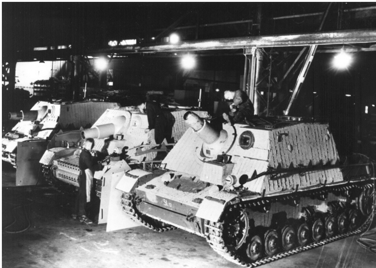
A line of completed Sturmpz on the pre-delivery inspection line at Stahlindustrie Werk, Duisburg; all have been coated with Zimmerit anti-magnetic mine paste. (Historyfacts)
